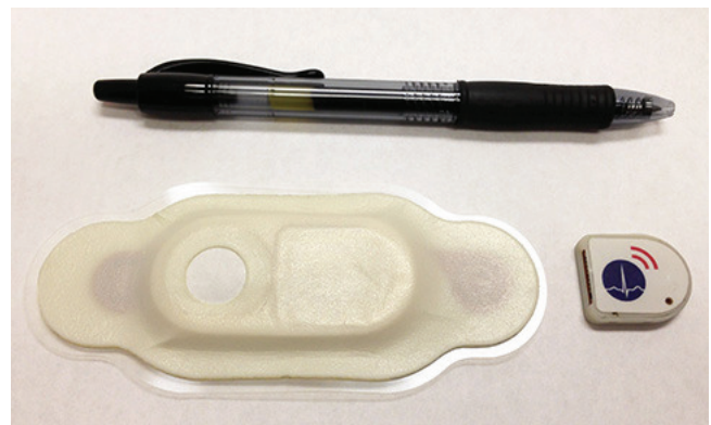
Fig. 1. Disposable Vital Connect patch sensor and reusable electronics module
